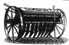
A positive FORCE-FEED, without clogging in any kind of commercial manure, sowing the same bulk of any PHOSPHATE with the same combination of gear. Quantity sown is regulated by a change of gear, in precisely the same manner as in sowing different quantities of grain.
