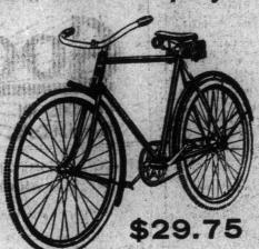
A thoroughly reliable Speedweil Bicycle that is remarkable for its low price. It's a bicycle that is suitable for either man or boy and one that will give years of service with reasonable care. It possesses the following specifications: Hercules coaster brake, roller chain, steel mud guards, extension handle bars, guaranteed double tube tires, and rattrap pedals. The frame is attractively finished with three coats of black enamel. Our leading value at ........... 29.75
