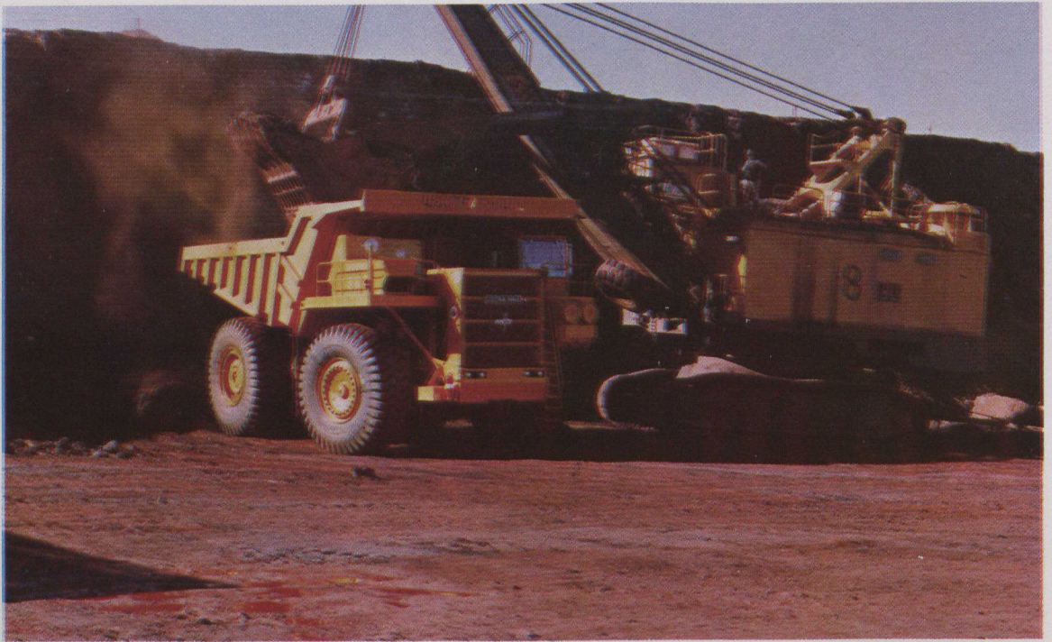
One of the Unitrig 36 electra haul 154.2 tonne payload trucks in use at one of the Hammersley Mines.
