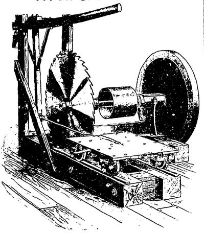
Timber when split with an axe will follow the grain of the wood, when split with a saw it is of course perfectly straight—no matter how winding the timber may be--and the first cut then is a perfect shingle; on this account alone a splitter will not saly save from 10 to 2 % of the timber, but will add about 5,000 shingles to each day's cut.
