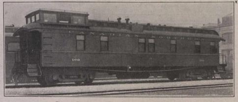
Fig. 1.-Canadian Northern Railway Dynamometer Car.
