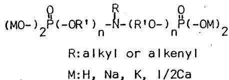
Salts(Na, K, Ca) of N-alkyl(or alkenyl)(C<sub>6~28</sub>)-N,N-di[polyoxyalkylene monophosphate]
