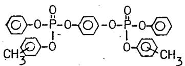
Phenylene bis(phenyl cresyl phosphate)
