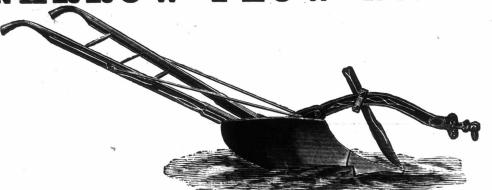
This is a cut of our Light General Purpose Narrow Plow No. 13. It is suitable for either heavy or light land. The mouldboard is of best Pittsburgh Soft Centre Steel, and is of such a shape and so hard a temper that it will clean in very sticky land where very many other plows will not.
