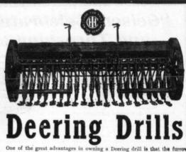
One of the great advantages in owning a Deering drill is that the furrow openers of the single disk, double disk and shoe drills are interc. angeable, consequently if you have need for any one of these styles of drills and have but one style of urrow opener you can purchase either or both of the other two styles and have a drill for all conditions of ground—hard and dry, trashy, muddy or well prepared seed bed.
