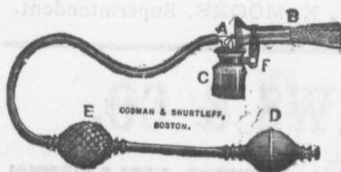
Fig. 5. Shurtleff's Atomizing Apparatus. Patented March 24, 1868.
