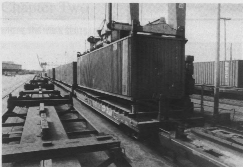
Overhead crane discharging container from rail car.
