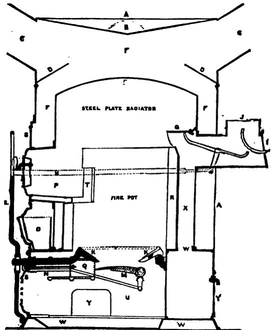
Marks a new era in the sanitary warming of our houses. The objections that have heretofore been urged against hot-air furnaces are entirely overcome in this apparatus. The vital point of superiority consists in covering the entire fire chamber and flues by an impervious drum of heavy steel plate, securely rivited. By this arrangement the escape or leakage of gases is an impossibility, while, by the system of flues used, the maximum quantity of heat is secured.
