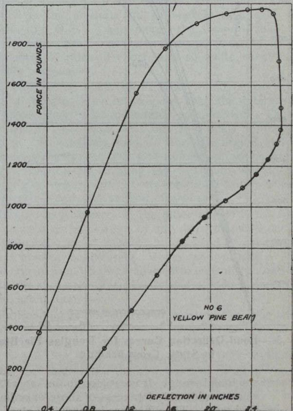
Fig. 4.—Impact Force-Deflection Curve for a Long-leaf Yellow Pine Beam Fractured but Retaining Considerable Resiliency. The Circles Space Off Equal Time-intervals
