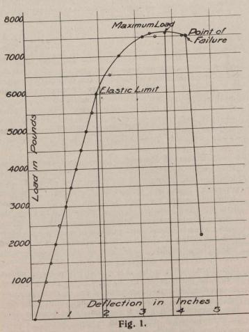
elastic limit was reached under a strain of 6,000 pounds and the maximum load at 7,580 pounds. Disks cut from the beam near the point of failure and dried in a steamheated copper kiln showed moisture content of 25%, 33% and 42; according to the distance they were taken from the surface.
