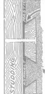
represents a cross section of wall, showing Plaster, Stucco, Stucco Board (note the Key holding Stucco) Asphalt, Mastic and
