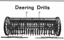
Deering drills for use in Western Canada have many exclusive features of peculiar value to Canadian farmers. The fact that the same frame can be equipped with single or double disk, or shoe furrow openers, is a point not to be over looked. It makes the Deering drill very adaptable—just the machine to buy for Western Canada. The rigid main frame is another important consideration.
