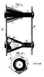
shells of bolts passing through said shells and the water-space, each bolt having a screw-threaded portion, a conical protector adapted to screw at its smaller end on each bolt so as to terminate between the ends of said bolt and each protector being adapted to bear tightly against the inner face of the outer shell, substantially as set forth.
