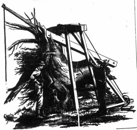
Will take out 20 to 50 stumps per day, depending on size. Three sizes. No. 1, capable of SIMON MILLER, Farmer. drawing any stump, \$120. No. 2, for stumps 2 feet 6 inches. \$90. No. 3, for 18 inch stumps, WILLIAM WARNOCK, Farmer \$70. The largest sizes will take out the smallest stumps, but they are constructed much stronger WILLIAM ADAMS, Farmer. and heavier.—Apply to PLUMMER & SON, Waggon Makers, London, or to W. WELD, DANIEL BROOKS, Farmer. Agricultural Emporium.
