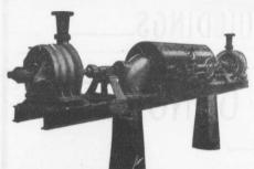
Two Worthington 3-Stage Turbine and McCormack Water Wheels, built for Port Arthur, Ont., Water Works, 1440 gal. per minute against 350 ft. head. WATER WORKS SYSTEMS INSTALLED
