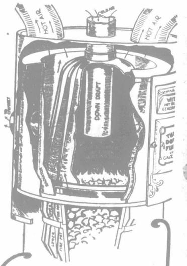
**The Down Draft Principle of Heating**
