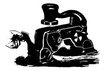
considerable skill is required to make good work, as the blow must be struck so as to divide the force evenly, otherwise a bad impression, (or, more properly speaking, "indentation,") is made, one side being cut deep into the wood or metal as the case may be, whilst the opposite side is barely touched. The unskilful use is also calculated to damage the tool.
