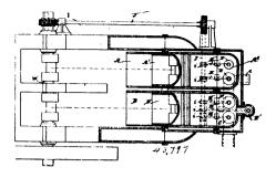
chamber in the end of the power cylinder, a communication passage with controlling valve between the adjacent end of the expansion cylinder and the combustion chamber, an air passage with controlling valve into the combustion chamber of the power cylinder, a gas inlet passage with controlling valve into the air passage, an air admission valve to the expansion cylinder and an exhaust valve therefrom, and means for operating said valves, substantially as herein described.
