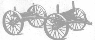
With metal wheels, is low and convenient for farm and general work. Made by skilled workmen, and of the best material. Guaranteed to carry four to five thousand pounds. Write for catalogue with full description of both Wheels and Wagons.
