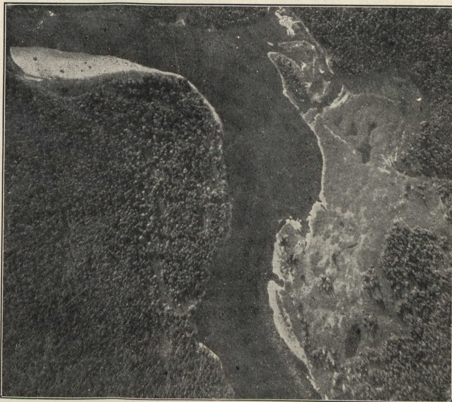
Showing how accurately timber can be photographed from the air by special aerial cameras. This shows a timber area with river and clearing. Hundreds of these pictures are taken and accurately fitted together to make a complete photographic mosaic.
