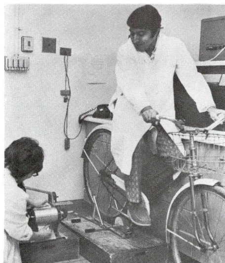
Passing dough through a roller run by a bicycle, a vehicle common in developing countries.
