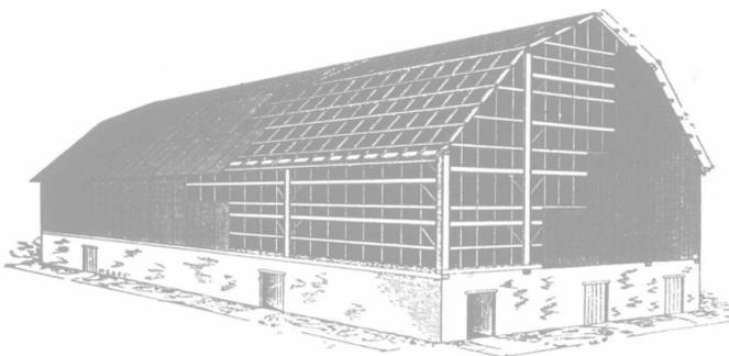
This cut shows an up-to-date Barn Construction, 40 feet x 70 feet, and the method of covering with Corrugated Sheets. The framework is light, as the corrugated sheets, when nailed in place, make the building very rigid. This drawing is made from actual plans and the barn has been built many times with splendid results.
