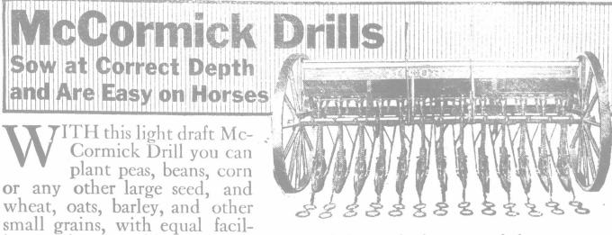
ity—without cracking or breaking any of the seed—because of the construction of the double-run force feed.
