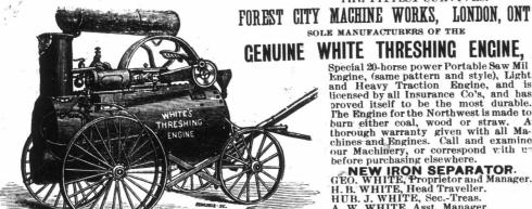
CENUINE WHITE THRESHING ENGINE, Special 20-horse power Portable Saw Mil Engine, (same pattern and style), Light and Heavy Traction Engine, and is licensed by all Insurance Co's, and has proved itself to be the most durable. The Engine for the Northwest is made to burn either coal, wood or straw. A thorough warranty given with all Machines and Engines. Call and examine our Machinery, or correspond with unbefore purchasing elsewhere.
