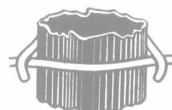
Front of post, showing post-hook gripping lateral wire.
