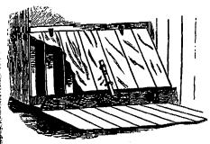
this made. The upright pieces prevent the pigs from getting into the trough, and it is easily cleaned from the outside of the pen.
