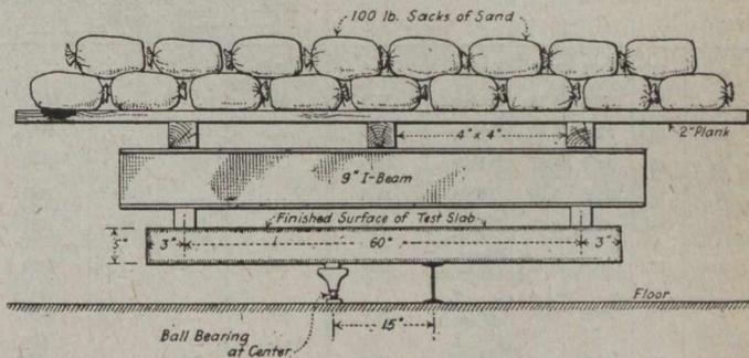
Fig. 1.—Method of Testing Slab.
