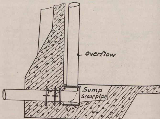
Fig. 5.—Overflow and Scour Pipe.
