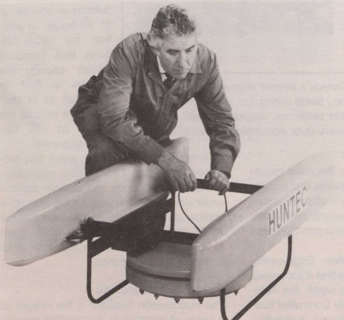
The SeaOtter is the newest high-resolution seismic sub-bottom profiler from Huntec, that features high-intensity acoustic pulse.
